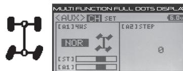
**REV: REVERSE (Tandem) Four Wheel Steering** - When Active, both the Front and Rear Steering will operate in Tandem.
