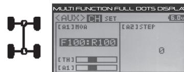
**REAR Throttle (BURN)** - When set to 0:100, power will only be distributed to the Rear motor. Power can be distributed proportionally between the Front and Rear motors from 0:100 to 99:100.
