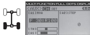
**FRONT Throttle (DIG)** - When set to 100:0, power will only be distributed to the Front motor. Power can be distributed proportionally between the Front and Rear motors from 100:0 to 100:99.
